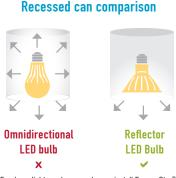
For down lights and recessed cans, install Energy Star® reflector LED bulbs. The light going upward from the omnidirectional bulbs can be wasted inside this fixture.
