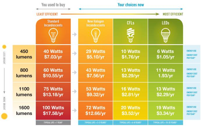
\*Rated life and energy cost per year based on 3 hours of use per day (energy cost per year based on Maritime Electric residential first block energy charge of \$0.1396/kWh and HST of 15%)
